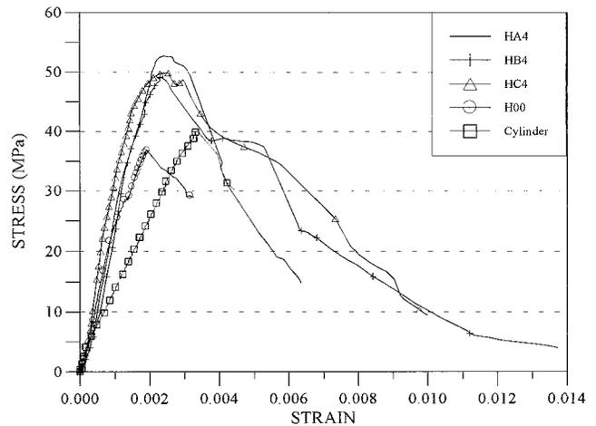
Fig. 10—Effect of configuration of lateral steel for specimens with higher-strength concrete.
