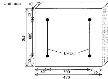
(b) a single wall panel cut from the hollow column
