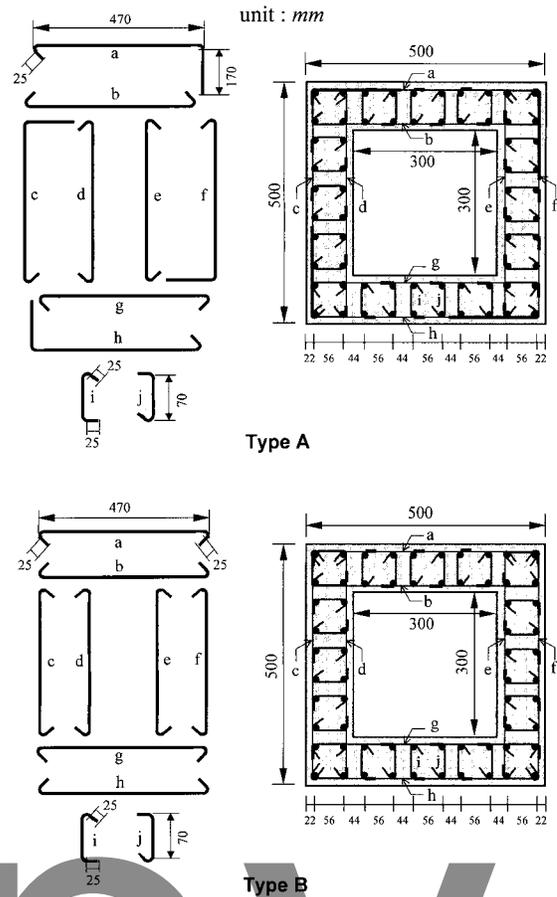
Fig. 4—Configurations of lateral steel (reinforcing bars  $f = 6$  mm, lateral steel  $f = 4$  mm).
