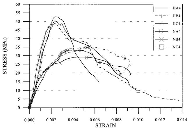
Fig. 9—Effect of concrete strength on stress-strain relationships.
