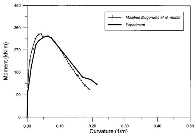
Fig. 19—Comparison of experimental results with modified Muguruma et al. model for moment-curvature curves of Specimen HB4.
