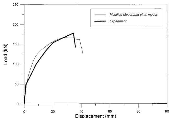
Fig. 20—Comparison of experimental results with modified Muguruma et al. model for load-displacement curves of Specimen HB4.
