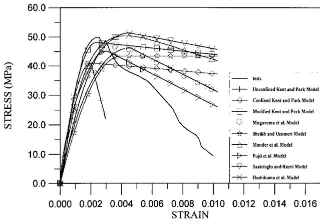
Fig. 12—Comparison of test results with nine analytical models for Specimen HC4.
