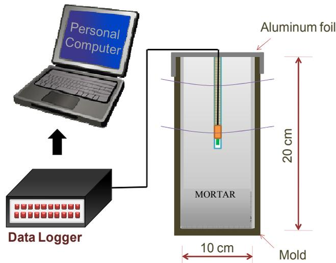
Figure 2. The setting of IRH measurement in sealed condition
