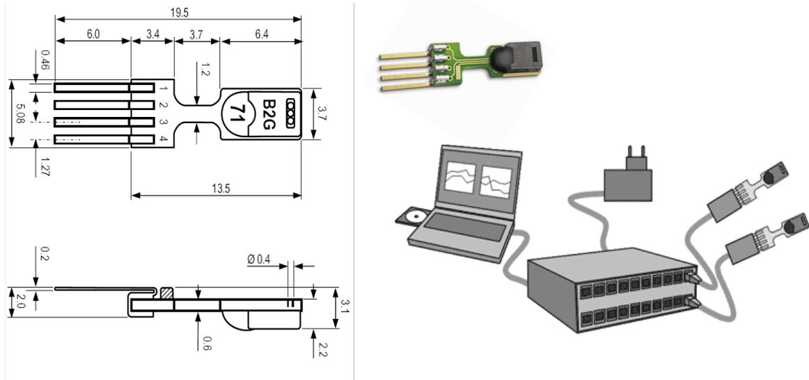
Figure 1. Sensor and IRH measurement set up
