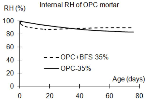
Figure 6. Internal RH of mortar with W/C ratio of 35%
