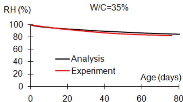
Figure 5. Internal RH comparison of analytical and experimental results
