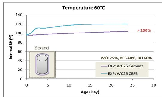
(c) Cement and BFS mortar at 60°C
