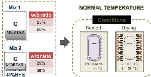
Fig 7 Test variables at normal temperature
