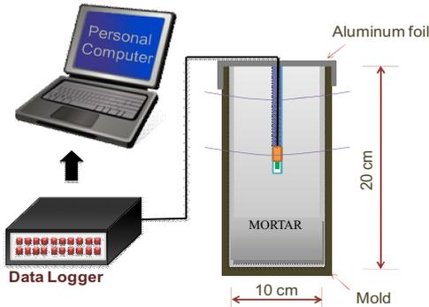
Fig 6 IRH measurement setting
