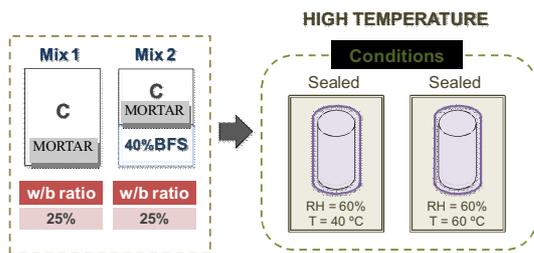
Fig 8 Test variables at high temperature
