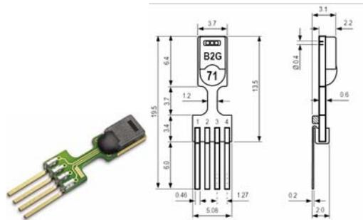
Fig 1 Capacitive sensor
