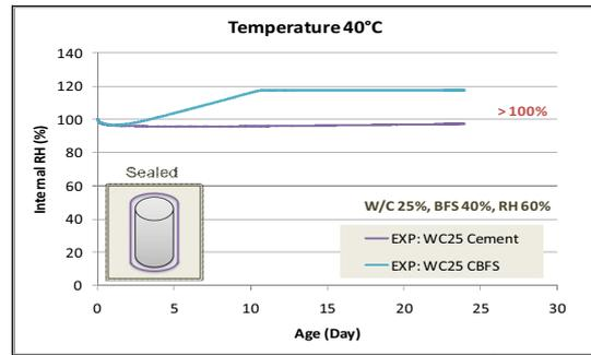
(b) Cement and BFS mortar at 40°C
