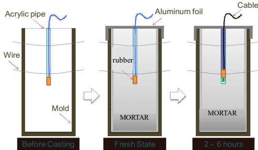
Fig 4 IRH Measurement proposed method
