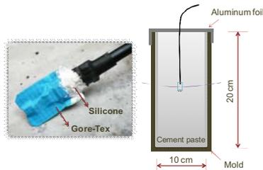
Fig 2 Sensor in fabric pouch embedded in mortar.
