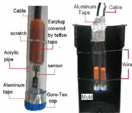
Fig 9 IRH measurement using double sensors
