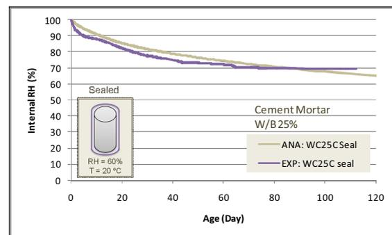
Fig 13 IRH of experiment result compared to analysis result by DuCOM
