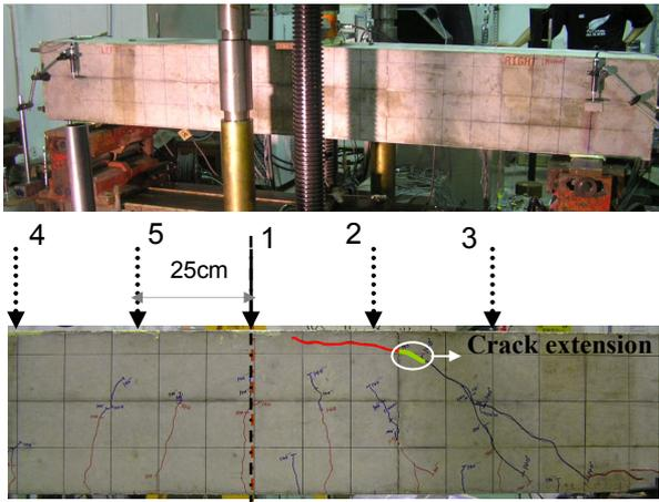
Fig. 8 Loading set up and Crack propagation at different loading points
