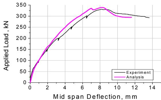
Fig.2 Static response, with web reinforcement
