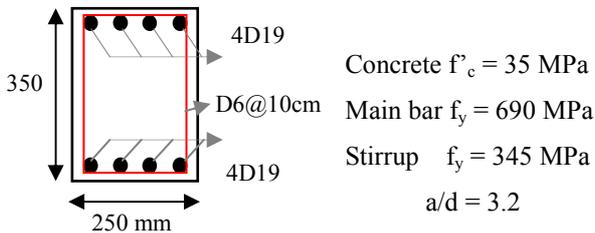
Fig1.Details of beam section with web reinforcement
