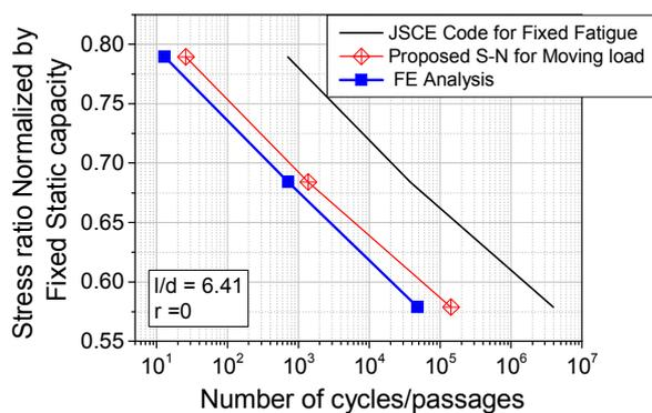
Fig.11 Proposed S-N diagram under moving load
