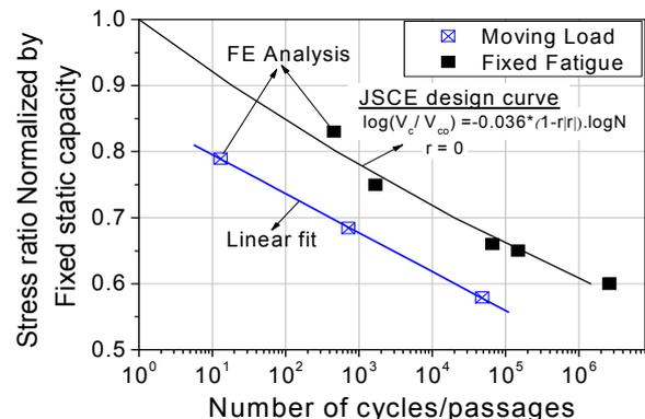
Fig.5 S-N diagram, beam with no web bar
