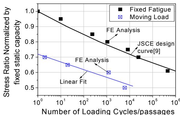
Fig.4 S-N diagram for beam with web bar
