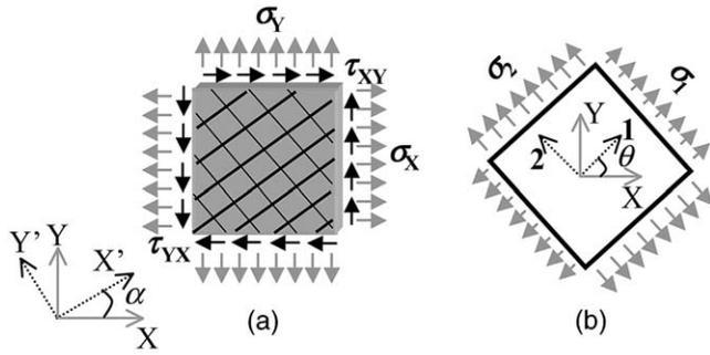
Fig. 2. RC Element subjected to in-plane stresses. (a) applied stresses; (b) principal directions of applied stresses.
