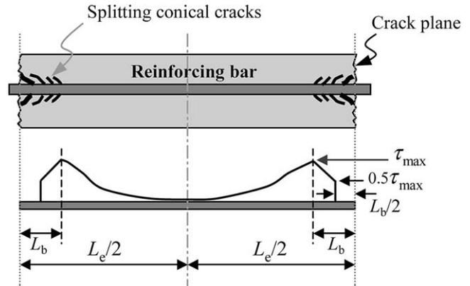
Fig. 5. Bond deterioration beside the crack surface.
