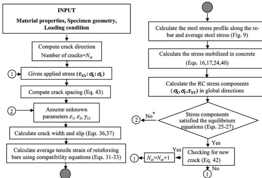
\* Note: The system of equations involving 3 equations (equilibrium equations) with 3 unknown parameters (concrete strains) is solved using an iterative method.
