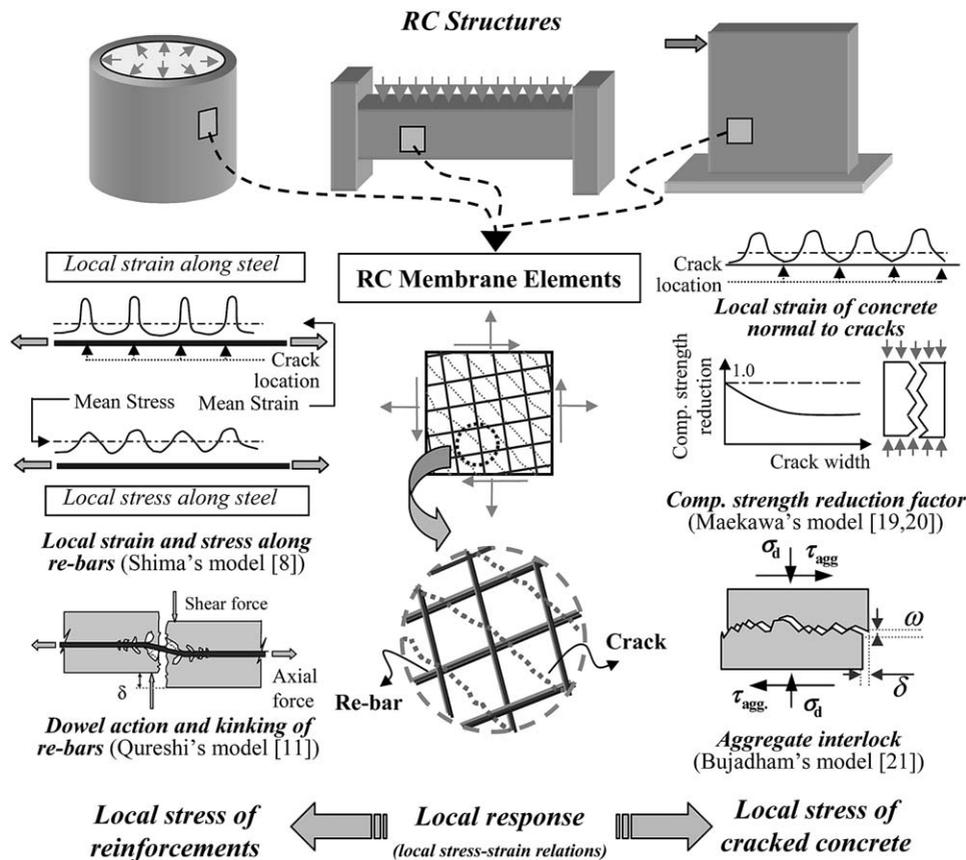
Fig. 1. Local stress transfer mechanism in RC membrane elements.
