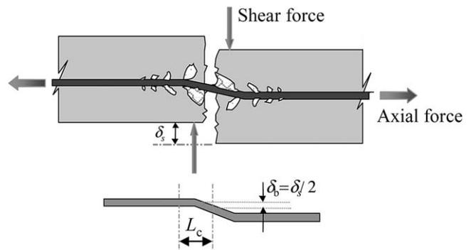
Fig. 6. Curvature of re-bar at the crack surface.
