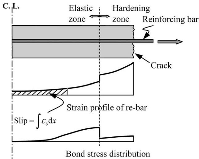
Fig. 4. Bond stress distribution and definition of slip.
