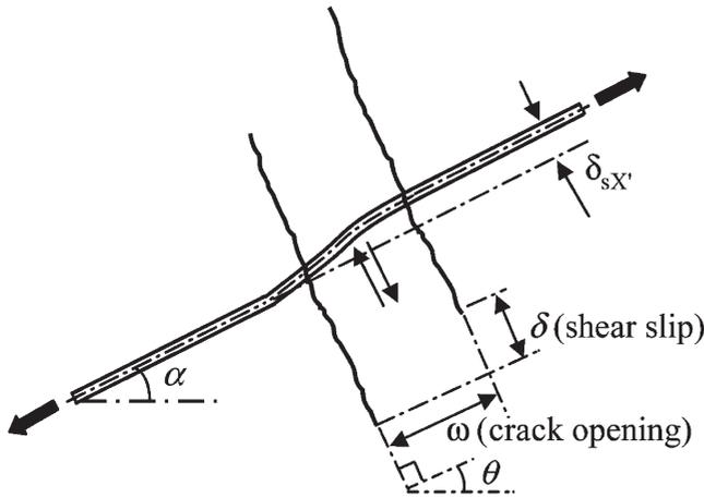
Fig. 12. Curvature of reinforcing bar due to opening and sliding.
