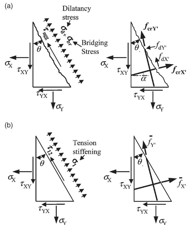
Fig. 10. Stress state of reinforcing bars and cracked concrete. (a) local stresses; (b) average stresses.
