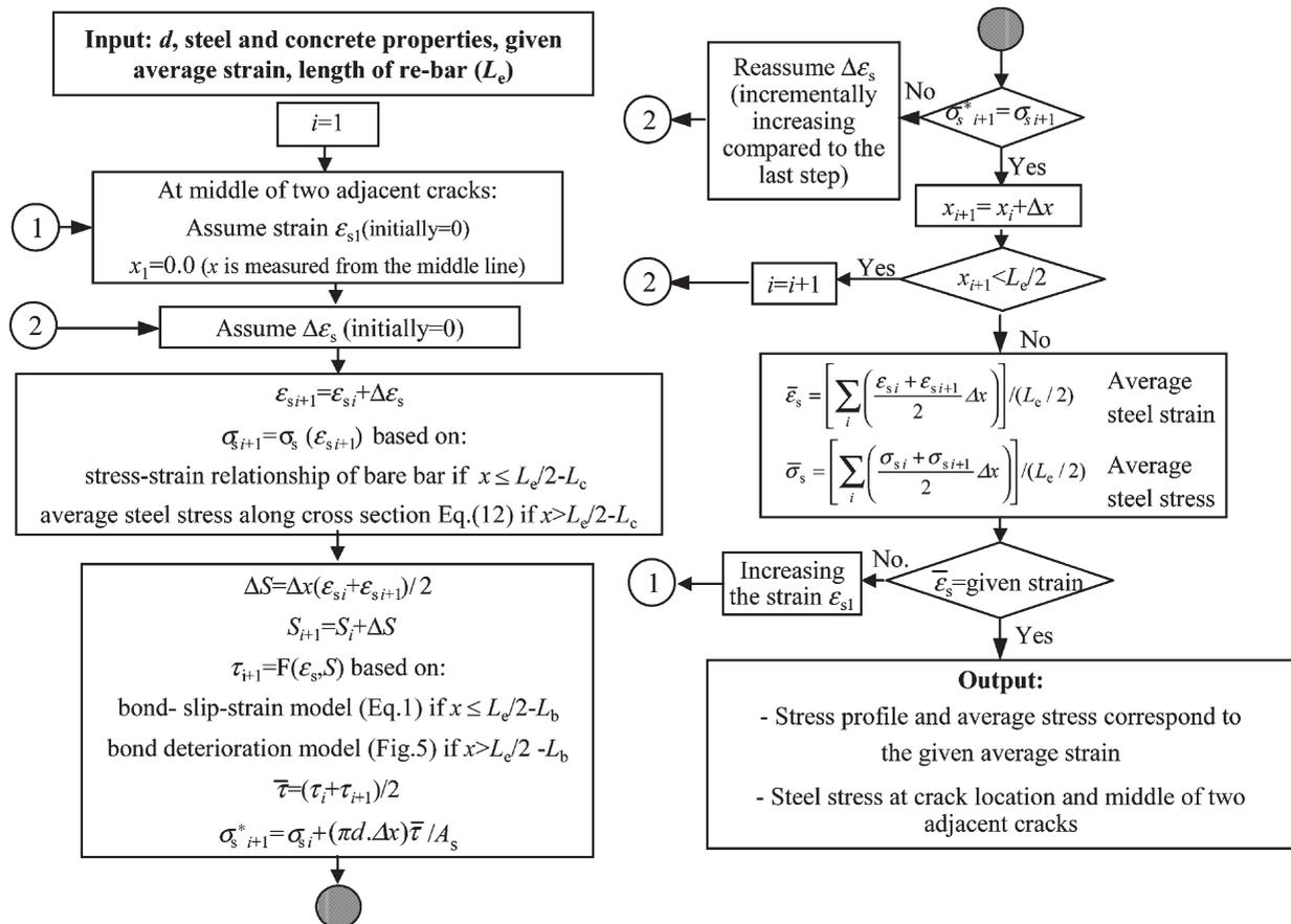
Fig. 9. Flowchart of computing stress-strain profile along the re-bars.
