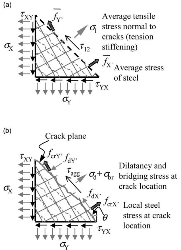
Fig. 3. State of stress of cracked concrete and reinforcing bars. (a) average stresses; (b) local stresses at crack location.
