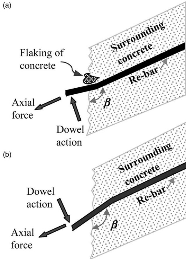
Fig. 7. Curvature influencing zone in the case of reinforcing bar oblique to the cracks. (a) re-bar push less confined surface; (b) re-bar push at right angle to the crack plane.
