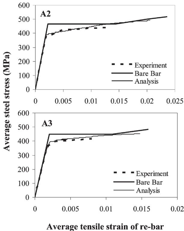
Fig. 17. Comparison between computed average stress-strain relationship of re-bars with experimental results (A2, A3) by Pang and Hsu [5].
