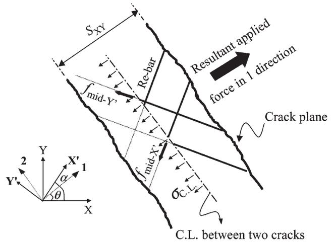
Fig. 13. Local tensile stress on centerline of two adjacent cracks.
