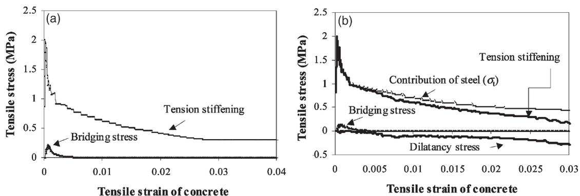
Fig. 18. The computed tensile stress components mobilized in RC domain. (a) panel A2; (b) panel B1.
