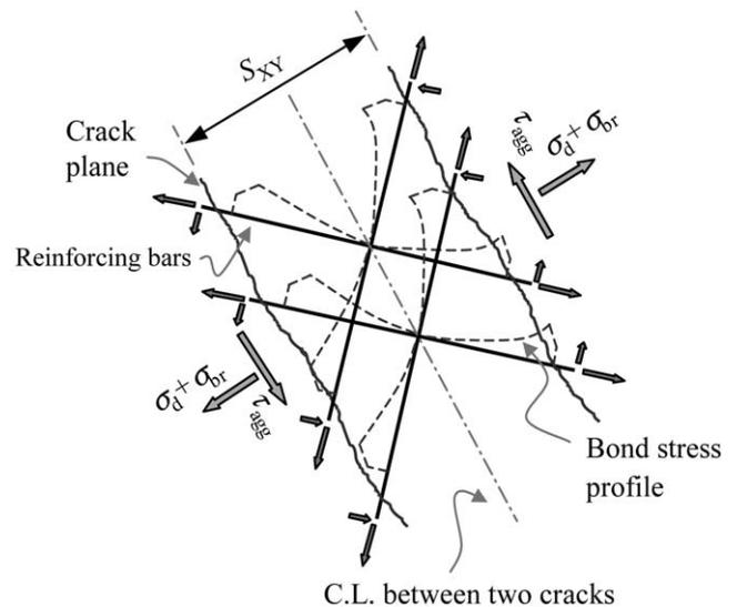
Fig. 11. The state of stress between two adjacent cracks.
