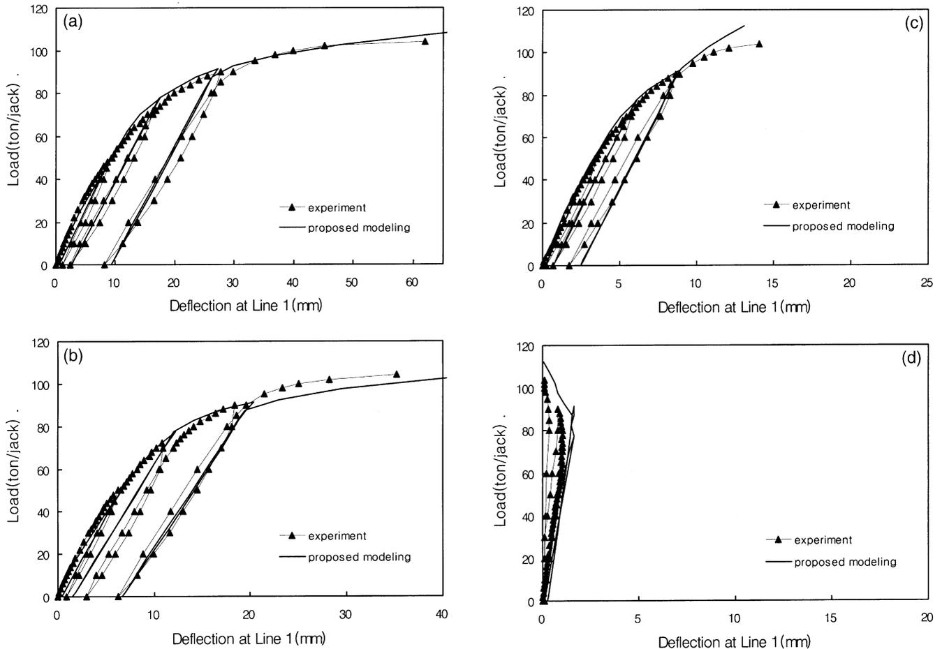
Fig. 17. Responses of second target bridge subjected to cyclic loading. (a) G1 girder; (b) G2 girder; (c) G3 girder; (d) G4 girder.
