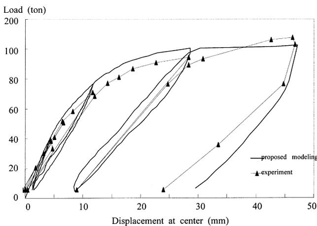
Fig. 16. Responses of first target bridge subjected to cyclic loading.
