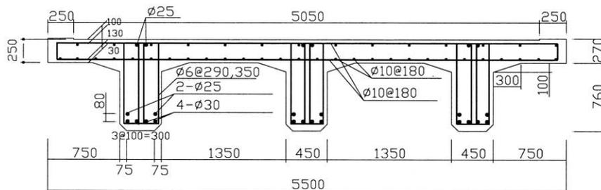
Fig. 1. Dimension of first target RC bridge (unit: mm).
