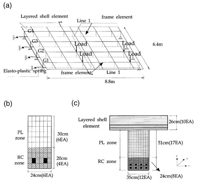
Fig. 13. Three-dimensional modeling of second target bridge. (a) Finite elements used for modeling; (b) discretization of transverse girder; (c) discretization of slab with longitudinal girder.
