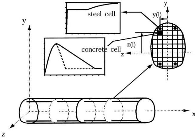
Fig. 11. Frame element with fiber technique.
