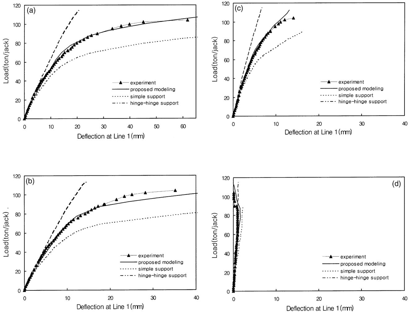
Fig. 15. Computed responses for different support conditions of second target bridge. (a) G1 girder; (b) G2 girder; (c) G3 girder; (d) G4 girder.
