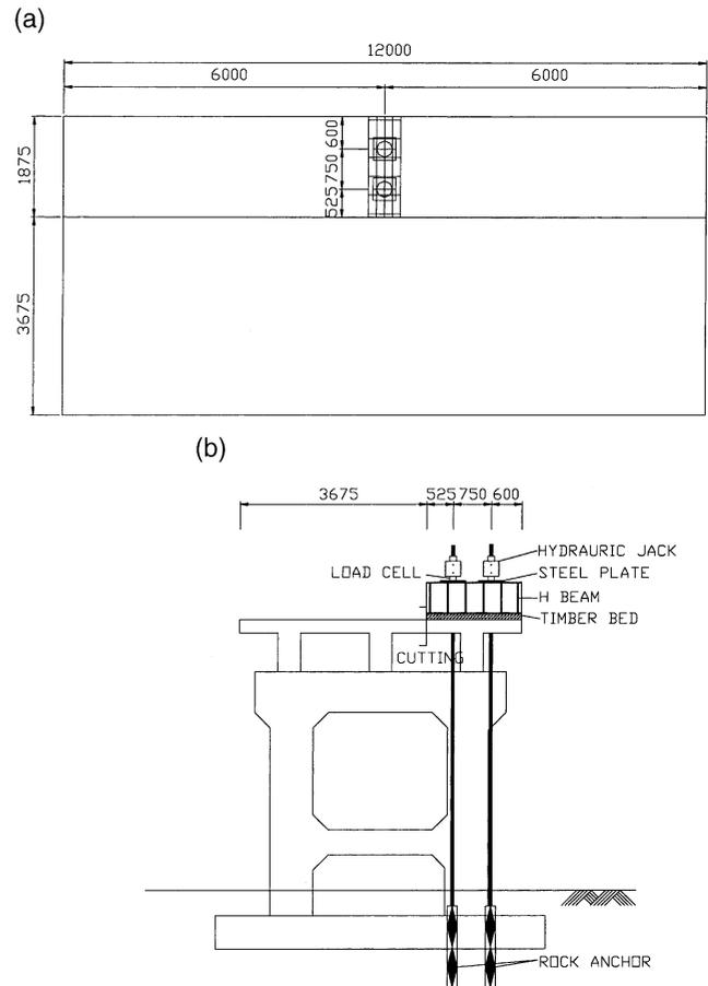
Fig. 4. Test set-up of first target bridge (unit: mm). (a) Plane view; (b) front view.
