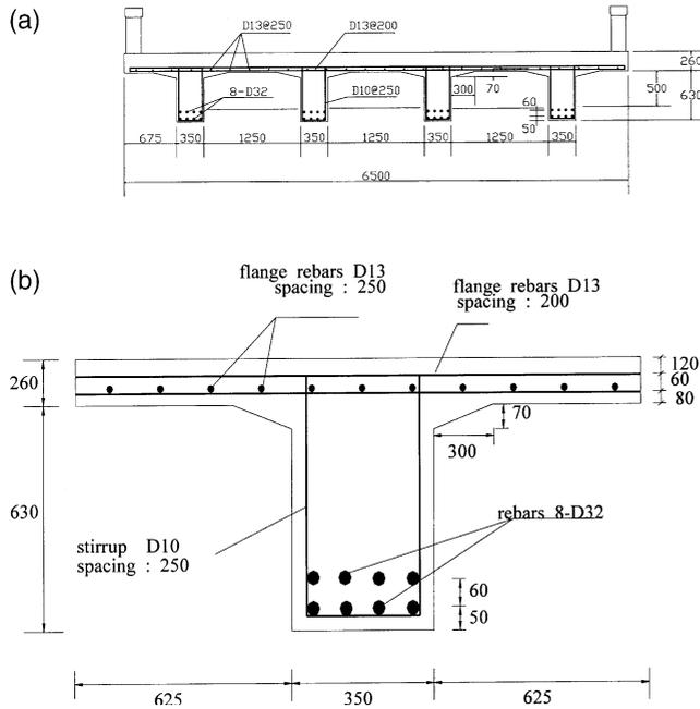
Fig. 3. Second target RC T-girder bridge (unit: mm). (a) Dimension; (b) reinforcement layout.
