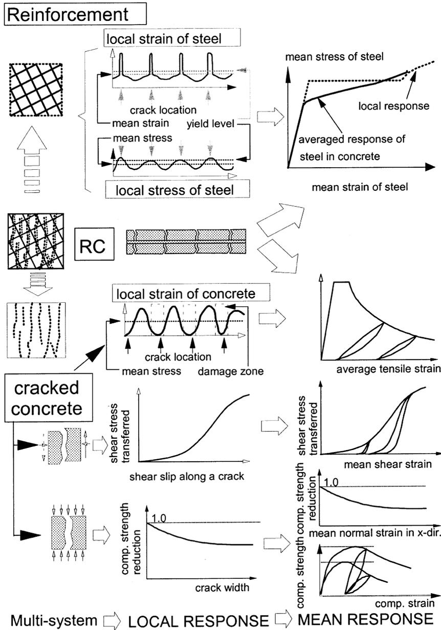
Fig. 8. Constitutive models of reinforced concrete.
