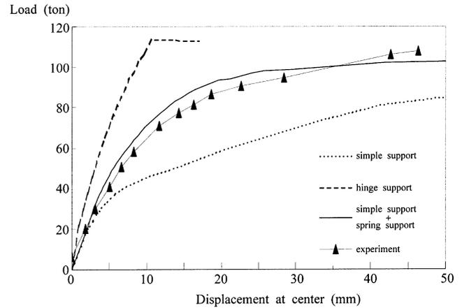
Fig. 14. Computed responses for different support conditions.
