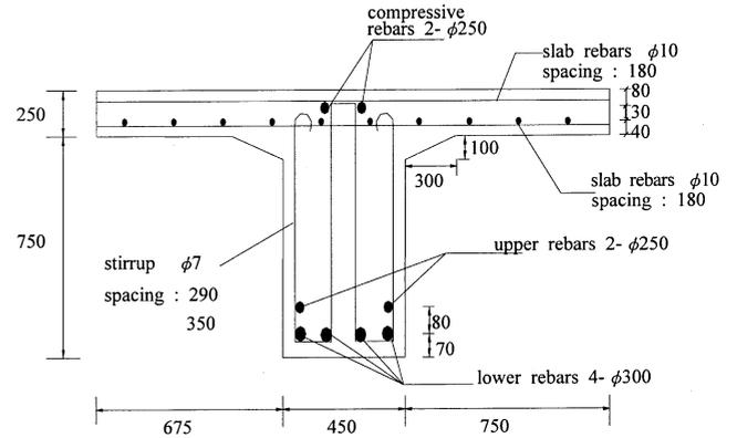
Fig. 2. Reinforcement layout of first target bridge section (unit: mm).
