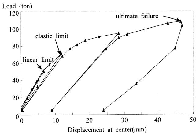
Fig. 6. Total applied load versus deflection response for first target bridge.
