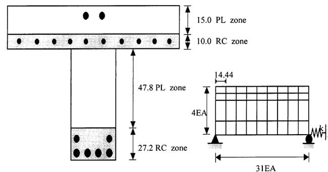
Fig. 10. 2D finite element modeling of first target bridge (unit: cm).
