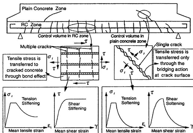
Fig. 9. Responses of concrete near and far from reinforcement.
