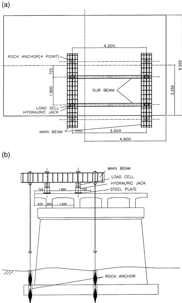
Fig. 5. Test set-up for second target bridge (unit: mm). (a) Plane view; (b) front view.
