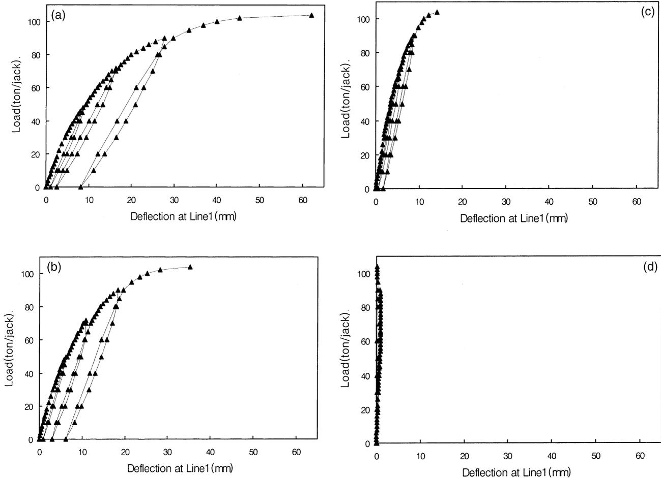
Fig. 7. Applied load versus deflection response for second target bridge. (a) G1 girder; (b) G2 girder; (c) G3 girder; (d) G4 girder.
