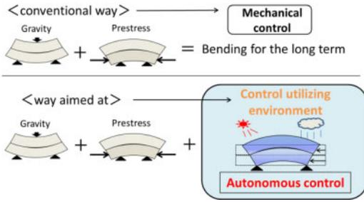
Figure 2. The concept of autonomous control of deflections.
