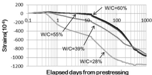
Figure 6. Simulated total strains of the each flange.
