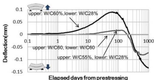
Figure 5. Simulated deflection of the specimen whose upper flange and bottom flange are composed of different water to cement ratios.
