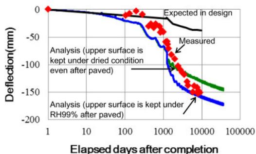
Figure 1. Analytical result of Tsukiyono bridge.
