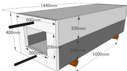
Figure 4. Shape and dimensions of the specimen.
