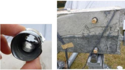
Figure 12. Left: small recorder of temperature and RH. Right: the way to measure the internal RH and temperature of both flanges.
