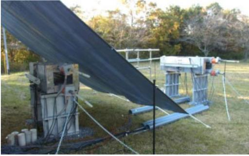
Figure 11. Experimental conditions. The left side is the PC beam with a roof and the right side is the PC beam without a roof and receives the influence of rainfall, solar-radiation.
