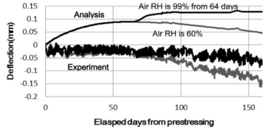
Figure 15. Analysis about deflections of a PC beam in rainy condition and a PC beam which doesn't take the rainy influence.
