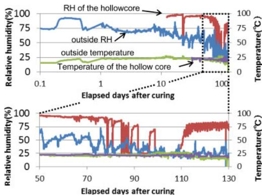
Figure 9. Temperature and relative humidity histograms, outside an inside of the hollow core.
