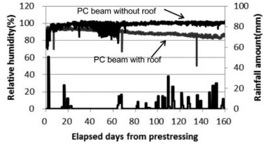
Figure 14. Internal RH of both upper flanges (the PC beam with a roof and the PC beam without a roof) and rainfall amount.
