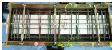
Figure 7. Arrangement of reinforcement: The diameter of deformed bars is 10 mm. 17 shear reinforcement bars and 14 axial reinforcement bars are arranged.
