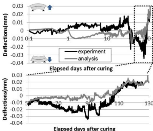
Figure 10. The computed and measured deflection.
