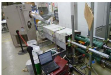
Figure 8. Experimental setup: The machine (left side of the specimen) is to control the temperature and humidity inside the hollow core.
