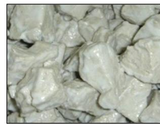
Epoxy-coated artificial lightweight gravel
