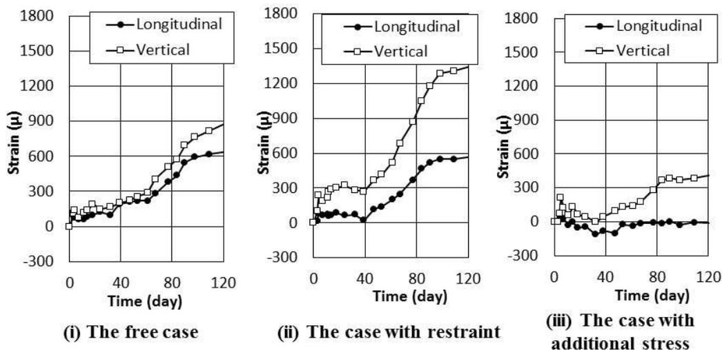
**Figure 4. Measured expansion in each restraint condition**
