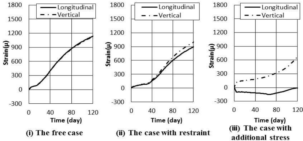
**Figure 5. Simulated expansion in each restraint condition**
