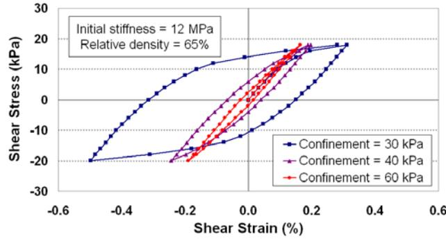
**Figure 1. Soil model under drained cyclic shear loading**
