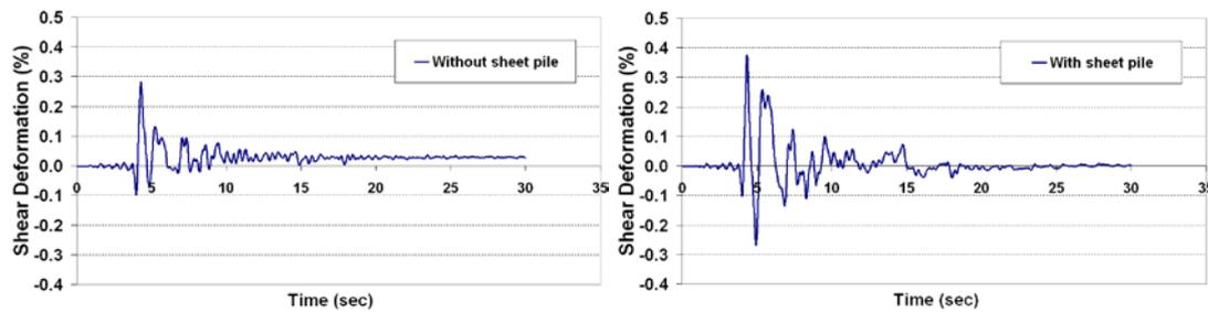
(a) Without sheet pile (b) With sheet pile
