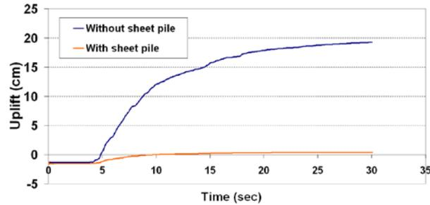
**Figure 7. Effect of sheet pile in reducing uplift**
