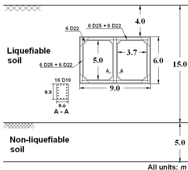
Figure 4. Soil-structure system geometry
