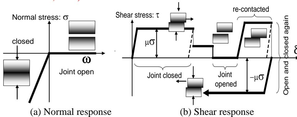
Figure 3. Normal and shear response of linear elastic interface model (Maekawa *et al*, 2008)
