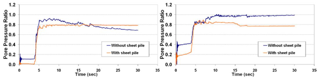
(a) 2.5 m below the tunnel (b) 1.5 m above the tunnel
