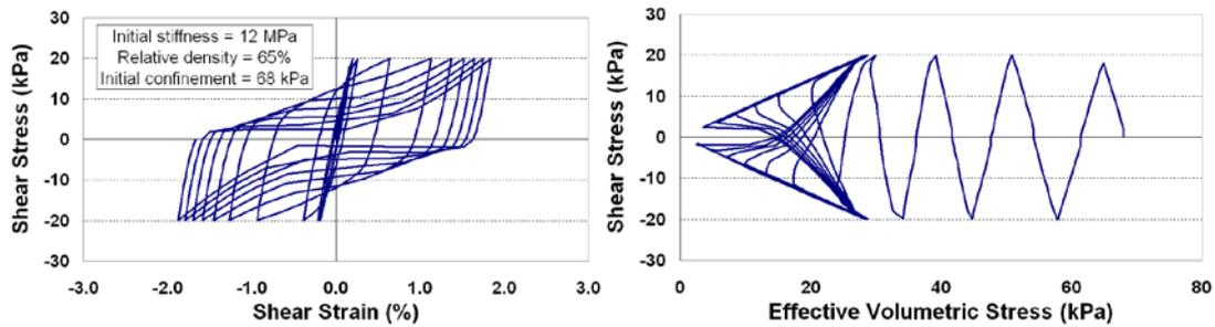
Figure 2. Soil model under undrained cyclic shear loading
