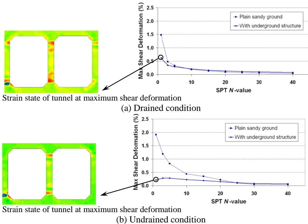
**Figure 6. Effect of soil stiffness on shear deformation**
