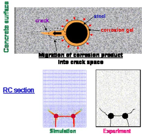
A mechanical effect of fractured stirrups due to corrosion or alkali-aggregate reaction was investigated. Significant reduction in shear capacity was found with no yielding of reinforcement when all web steel anchorage was incomplete near the tensile steel. The longitudinal cracks were formed ultimately along the tensile steel where the cut-off of web reinforcements lies due to insufficient anchorage performance at the fractured portion.
